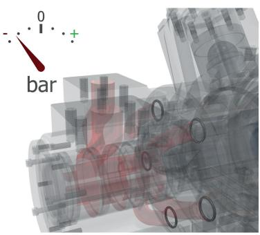
Cavitation can occur due to many different factors. Although it is not possible to make the HMC motor resistant to cavitation, certain features can be added to improve the motor's resistance to short periods of lost port pressure.
