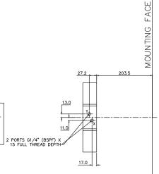
MOUNTING INTERFACE FOR DIRECTIONAL CONTROL VALVE\* TO: ISO 4401 SIZE 03/ANSI B93,7M SIZE D03 \*DISPLACEMENT SELECTOR VALVE IS NOT SUPPLIED WITH MOTOR; SPECIFY & ORDER SEPARATELY
