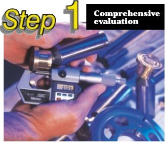
Each component is inspected/checked for finish and clearance. Failure modes are reviewed to identify the root cause of failure.
