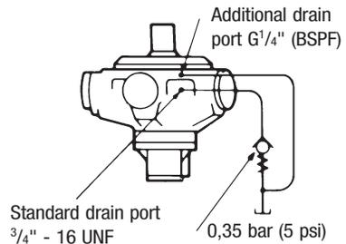
An additional G<sup>1</sup>/<sub>4</sub>" (BSPF) drain port in the front mounting flange is provided when the “V” (shaft vertically upwards) designator is given after the shaft type letter in position **3** of the model code. This additional drain should be connected into the main motor casing drain line downstream of a 0,35 bar (5 psi) check valve to ensure lubrication of the upper bearing, see above diagram.
