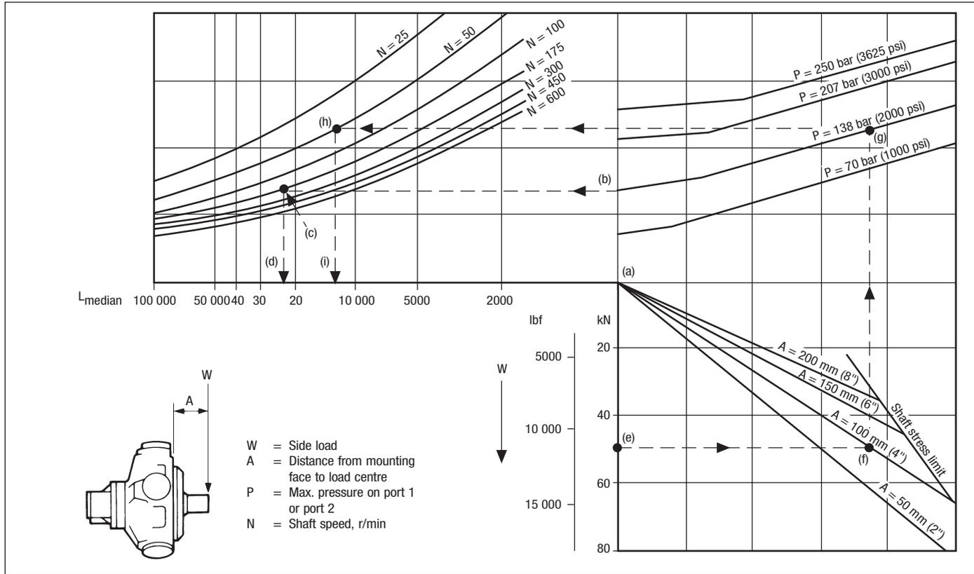
The nomograph allows the median bearing life to be determined for conditions of:
