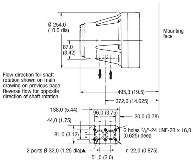
▲ Ø 32 (1.25 dia), with recess for 38,1 (1.50) i/d x Ø 3,53 (0.139 dia) section O-ring
