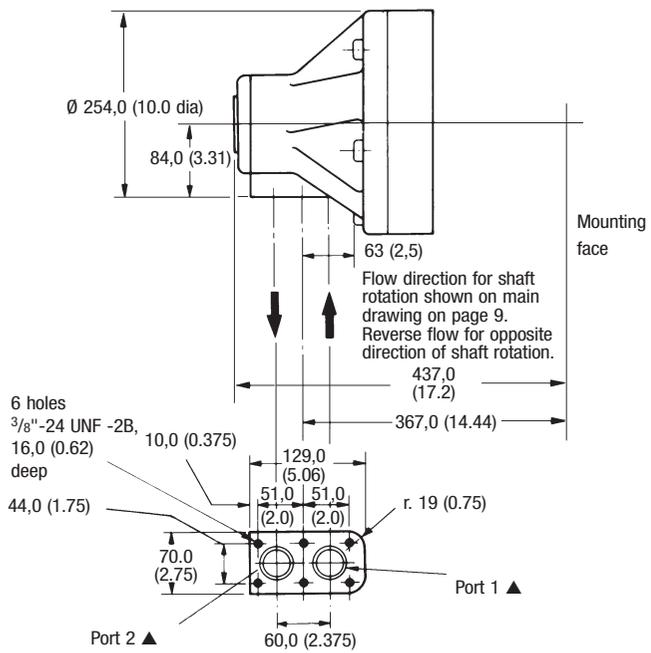
▲ Ø 28 (1.125 dia), with recess for 31,0 (1.22) i/d x Ø 4 (0.157 dia) section O-ring
