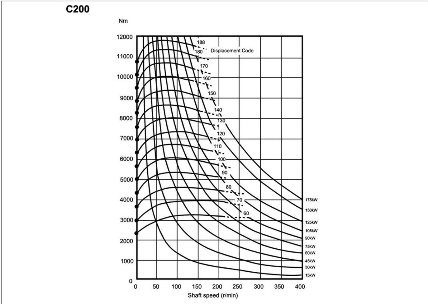
The torque curves indicate, for each displacement, the maximum output torque of the motor with an inlet pressure of 250 bar (3626 psi) and zero output pressure. High return line pressures will reduce the torque for any given pressure differential.
