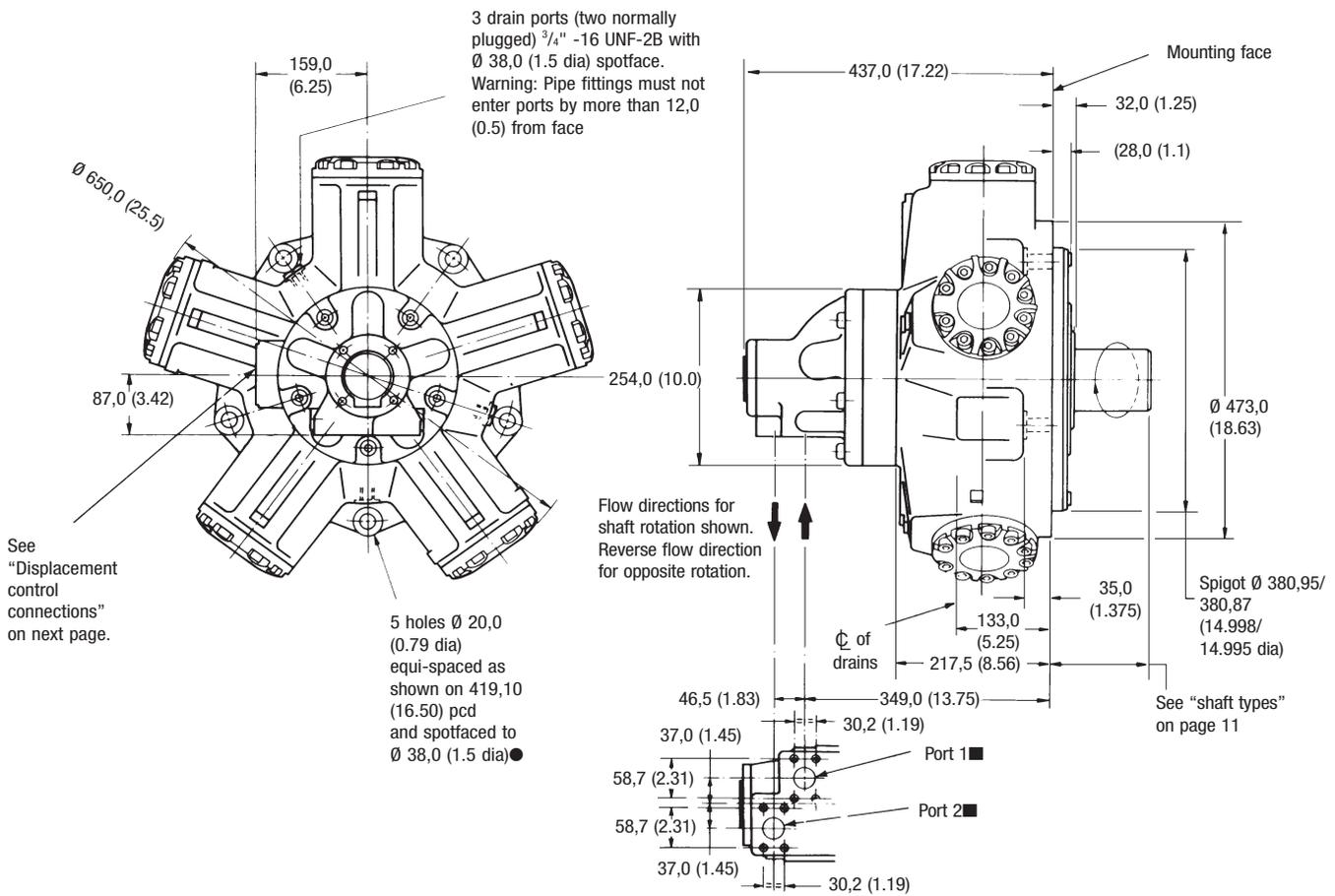
● Suitable for M20 or 3/4" bolts. Maximum reaming diameter 21,0 (0.83) (for fitted bolt); see "Installation Data".
