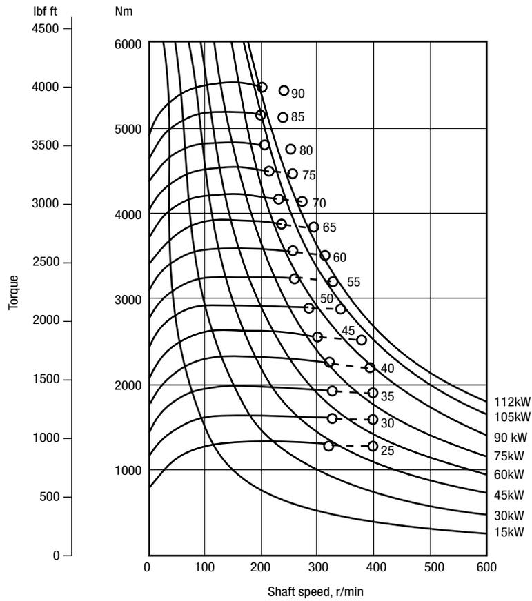
The torque curves indicate, for each displacement, the maximum output torque of the motor with an inlet pressure of 250 bar (3626 psi) and zero output pressure. High return line pressures will reduce the torque for any given pressure differential.
