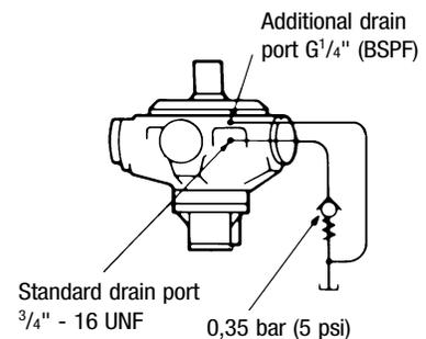
An additional G<sup>1</sup>/<sub>4</sub>" (BSPF) drain port in the front mounting flange is provided when the “V” (shaft vertically upwards) designator is given after the shaft type letter in position **3** of the model code. This additional drain should be connected into the main motor casing drain line downstream of a 0,35 bar (5 psi) check valve to ensure lubrication of the upper bearing. See above diagram.
