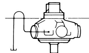
Use any drain position. The drain line should be run above the level of the uppermost bearing; if there is risk of syphoning then a syphon breaker should be fitted.
