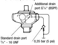
Specify "V" at model code position (3) for extra drain port, G<sup>1</sup>/<sub>4</sub>" (BSPF). Connect this port into main drain line downstream of a 0,35 bar (5 psi) check valve to ensure good bearing lubrication. Piping arrangement must not allow syphoning from the motorcase. Where this arrangement is not practical, please consult Kawasaki.
