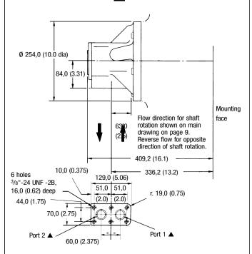
▲ Ø 28 (1.125 dia), with recess for 31,0 (1.22) i/d x Ø 4 (0.157 dia) section 0-ring
