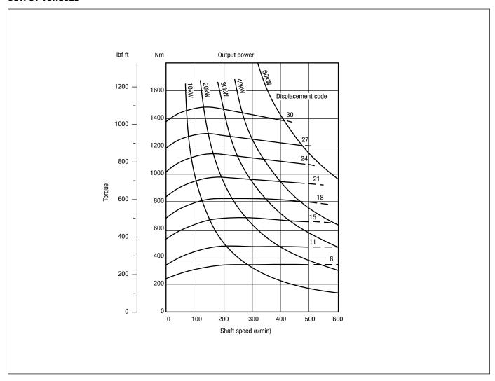
The torque curves indicate, for each displacement, the maximum output torque of the motor with an inlet pressure of 250 bar (3626 psi) and zero output pressure. High return line pressures will reduce the torque for any given pressure differential.
