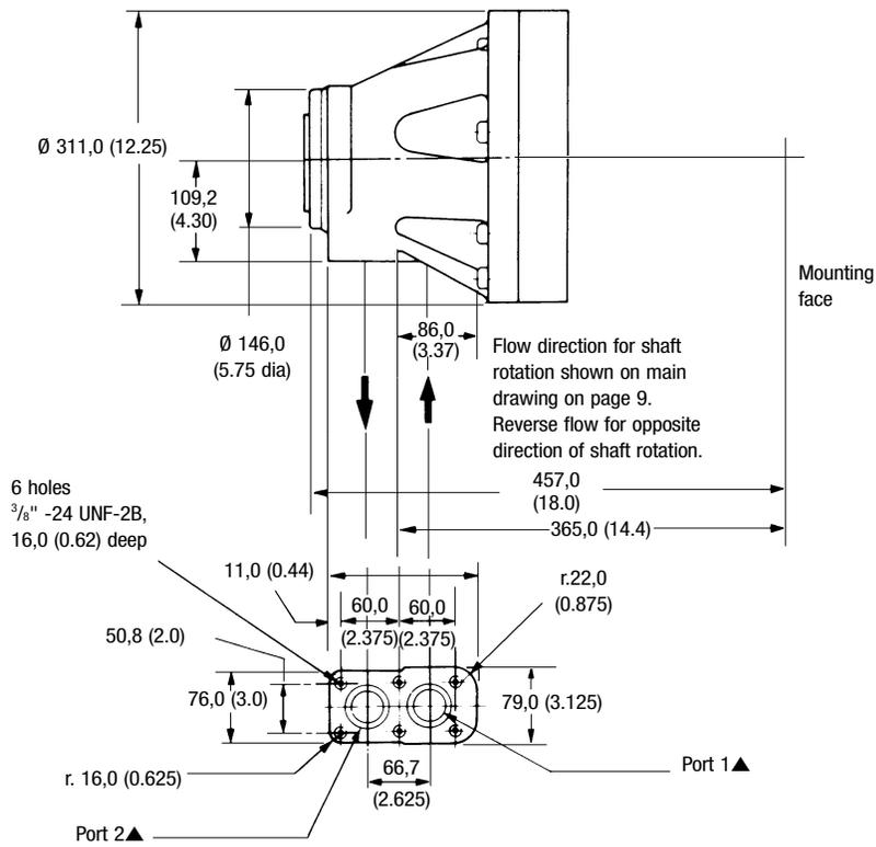
▲  $\varnothing 35,0$  (1.325 dia), with recess for 38,1 (1.5) i/d x  $\varnothing 3,53$  (0.139 dia)
