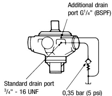
An additional G<sup>1</sup>/<sub>4</sub>" (BSPF) drain port is provided in the front cover when the “V” (shaft vertically upwards) designator is given after the shaft type letter in position **3** of the model code. This additional drain should be connected into the main motor casing drain line downstream of a 0,35 bar (5 psi) check valve to ensure lubrication of the upper bearing, see above diagram.
