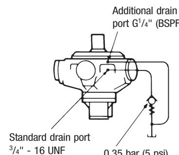
An additional G1/4" (BSPF) drain port is provided when the "V" (shaft vertically upwards) designator is given after the shaft type letter in position 3 of the model code. This additional drain should be connected into the main motor casing drain line downstream of a 0,35 bar (5 psi) check valve to ensure lubrication of the upper bearing, see above diagram.
