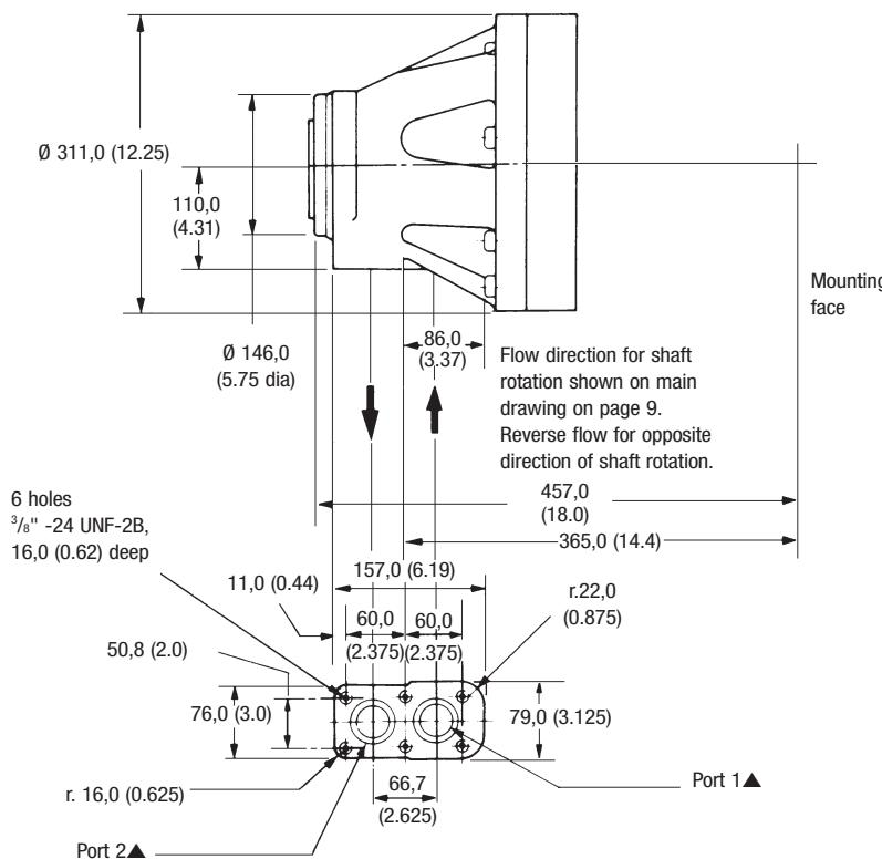
▲ Ø 35,0 (1.325 dia), with recess for 38,1 (1.5) i/d x Ø 3,53 (0.139 dia)
