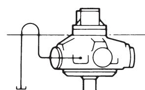
Use any drain position. The drain line should be run above the level of the uppermost bearing; if there is risk of syphoning then a syphon breaker should be fitted.
