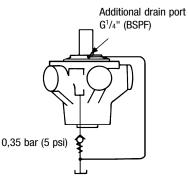
An additional G¹/4" (BSPF) drain port is provided when the "V" (shaft vertically upwards) designator is given after the shaft type letter in position ⑤ of the model code. This additional drain should be connected into the main motor casing drain line downstream of a 0,35 bar (5 psi) check valve to ensure lubrication of the upper bearing, see above diagram.
