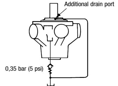
An additional drain port is provided when the “V” (shaft vertically upwards) designator is given after the shaft type letter in position **3** of the model code. This additional drain should be connected into the main motor casing drain line downstream of a 0,35 bar (5 psi) check valve to ensure lubrication of the upper bearing.
