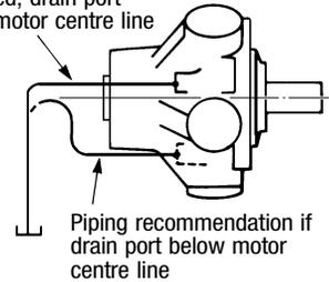
The motor should be installed with the drain port above the shaft centre line to ensure adequate lubrication of the bearings. When this is not possible and the drain port is positioned below the shaft centre line, the drain line should be run to at least the level of the shaft centre line; see above diagram.
